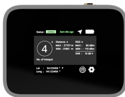
Figure 2: RAK10701-L front view with an LCD screen
