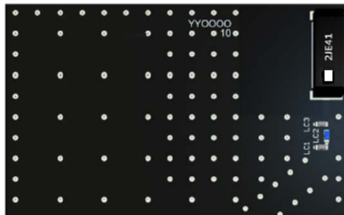
3D View of matching components and recommended values (LC1=3.9 pF, LC2=10 pF, LC3=DNP)
