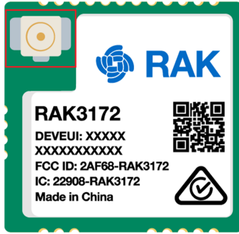
Figure 3: IPEX Connector of RAK3172 for LoRa Antenna
