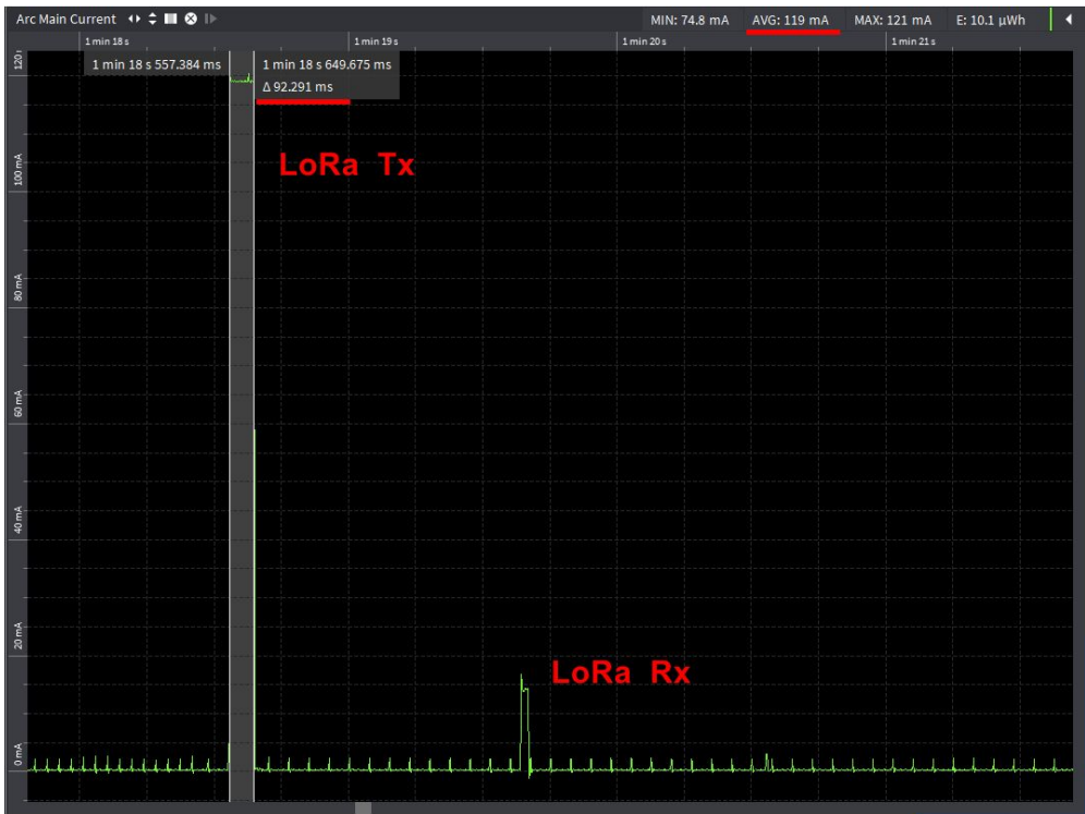
Figure 4: Oscilloscope Screen Capture of LoRa Packet Sending
