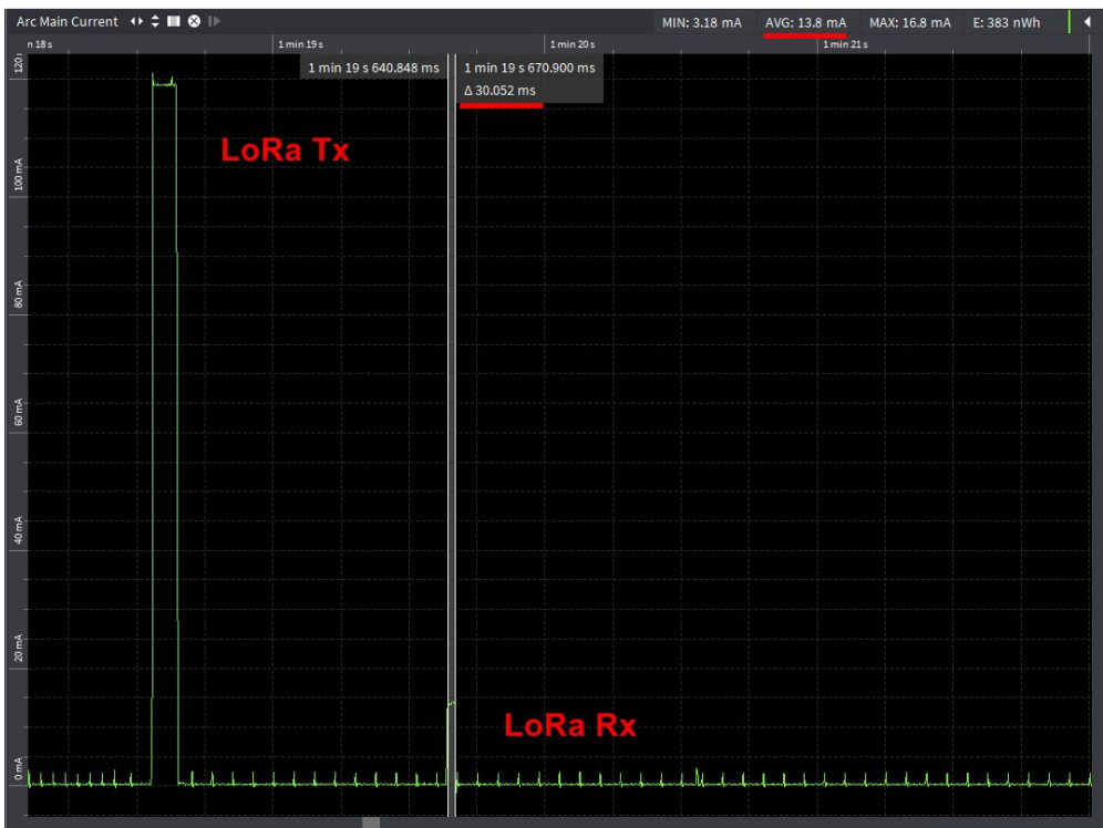
Figure 5: Oscilloscope Screen Capture of LoRa Packet Receiving
