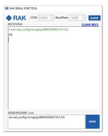
Figure 59: Configuring P2P in both RAK4270 Module
