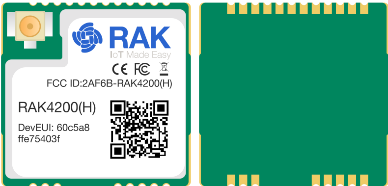
Figure 1: RAK4200 WisDuo LPWAN Module Front and Back View
