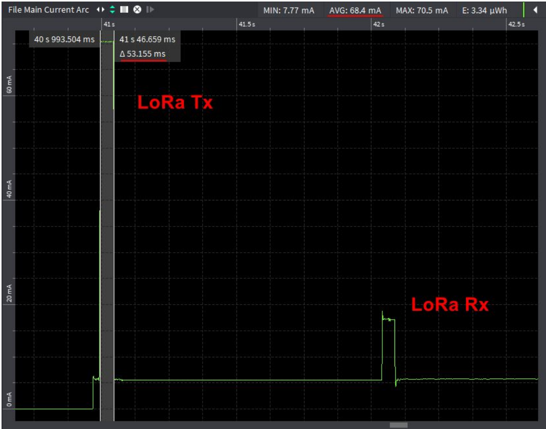
Figure 4: Oscilloscope Screen Capture of LoRa Packet Sending
