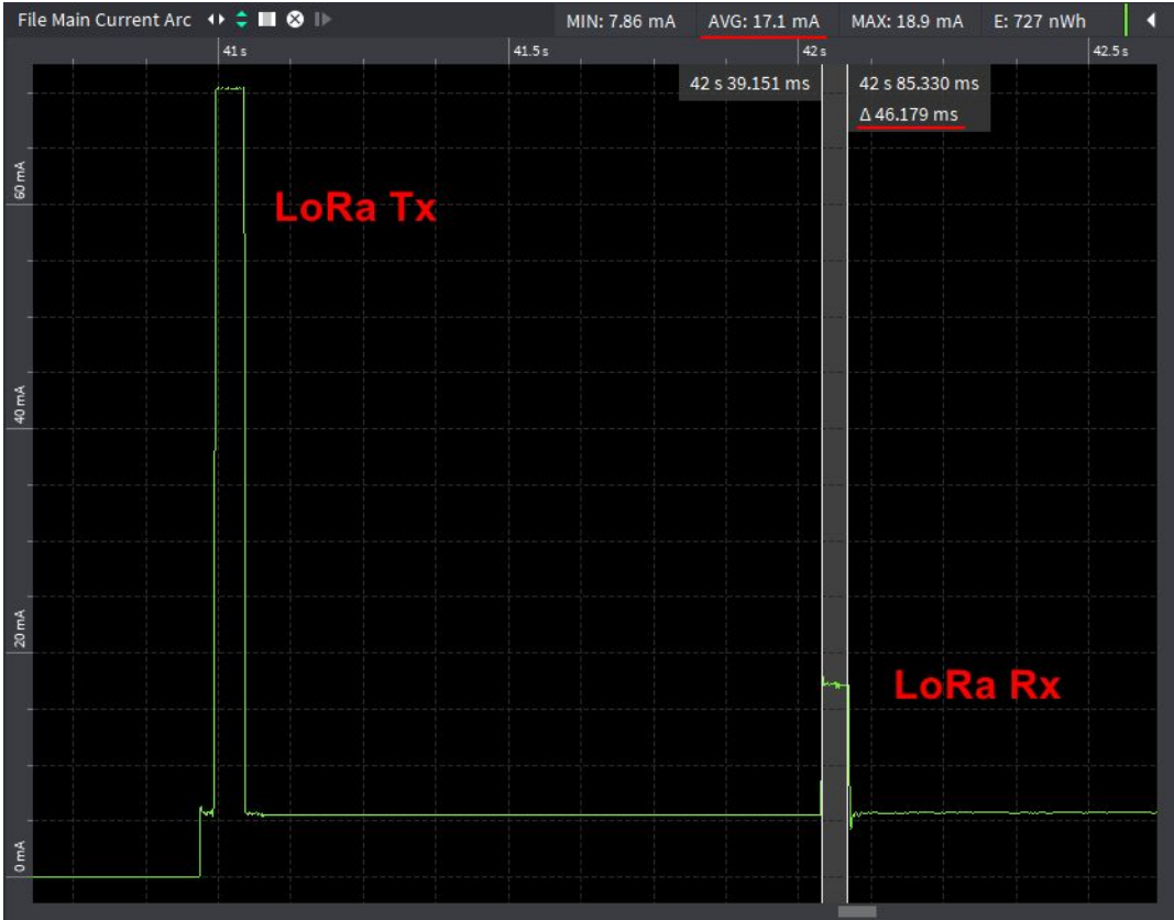
Figure 5: Oscilloscope Screen Capture of LoRa Packet Receiving
