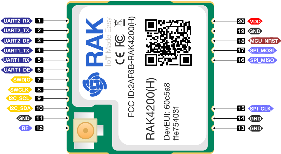
Figure 3: Pinout for RAK4200
